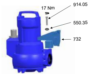
Fig. 10: Fastening the claw for single guide rail
